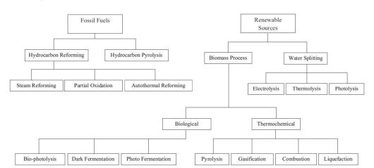
Figure 2-1: HYDROGEN PRODUCTION PROCESSES (Nikolaidis and Poullikkas 2017)
