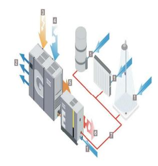
1) Cold water 2) Compressed air 3) Electric power 4) Air 5) Oil circuit 6) Energy recovery 7) Warm water
