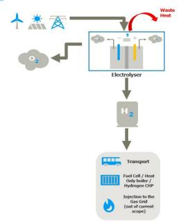
Figure 2-2: GREEN HYDROGEN PRODUCTION PROCESS
