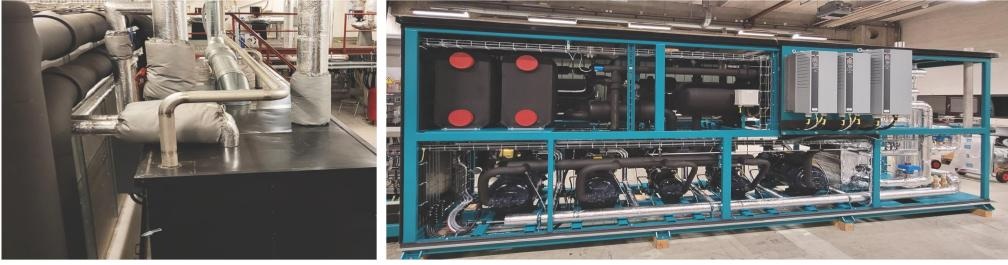
YEAR: 2021 MODEL: H1000-WW APPLICATION: Water-to-water heat pump CAPACITY (HEAT): 900 kW (-4,5°C evaporator, 30/55°C hot water) HEAT SOURCE: Ground source boreholes COP: 3,58
